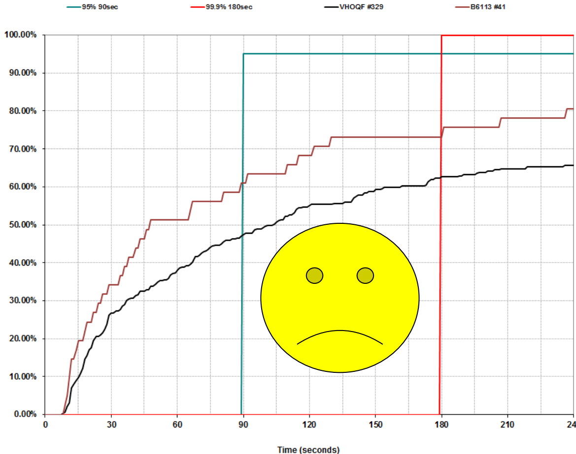
A388 VHOQF No SATCOM 24 Nov 15 - 14 Dec 15 A332 B6113 No SATCOM 18 Dec 15 Actual ADS-C HFDL Performance against RSP180 standard KZAK, NZZO, YBBB, YMMM FIR
